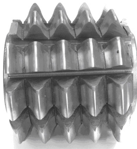
Figure 7: Real hobbing cutter for machining of convex-concave gearing
