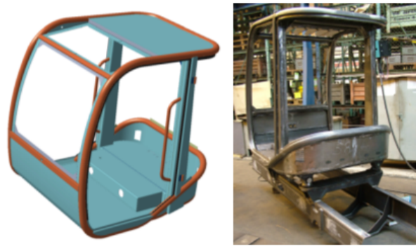
Figure 2: 3D model and the real body in white of cab
